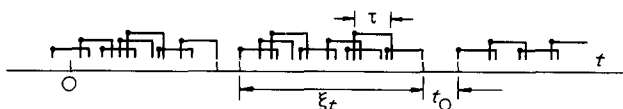
Figure 1 The history of a chain represented in a one-dimensional time diagram. Each segment indicates a crosslink, acquired at the time where the segment starts (filled circles) and broken at the time where it ends
